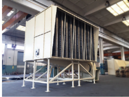
Inertial Filters and Bleed Fans
